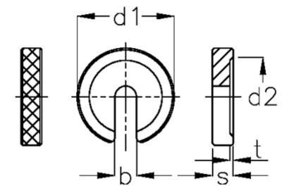
$\begin{array}{lll} b & = 8.3 \\ d1 & = 28 \\ d2 & = 21 \\ For bolt = M8 \\ s & = 7 \\ t & = 1.0 \\ \end{array}$
